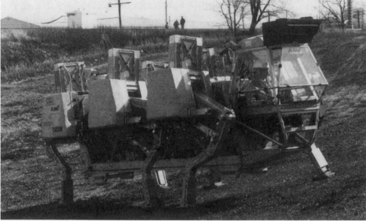
FIGURE 1.10. The OSU ASV. An example of a six-legged walking machine (courtesy of Prof. K. Waldron. Reproduced with permission of The MIT Press.)
